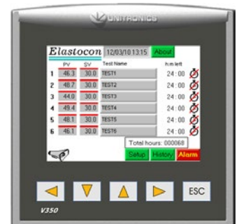
All ageing ovens have a touch screen control utilising a micro PLC.
