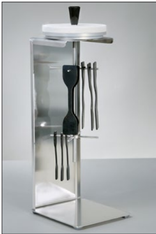
Stand EB 01.01 , stand to support the sample holder while mounting test pieces for ageing.
